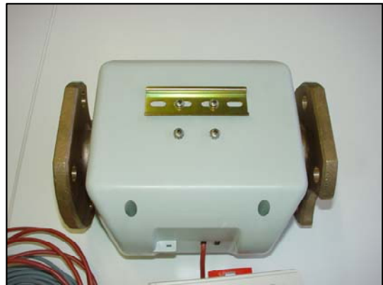
Fig. 2: PolluFlow – integrator removed
