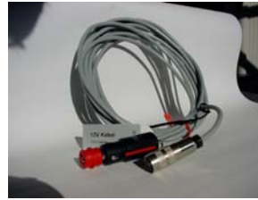
A 12 V / 220 V plug for external power supply of the gsm modem or charging the accus of the gsm modem.
