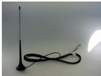
900 Mhz antenna with a plug for the connection to the gsm modem.
